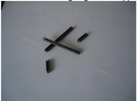
What needs to be done is to drill partially (**not right through**) into the lower half of the hinge, hammer in the roll pin, cut/grind off the excess pin and paint over. Job done and now the hinge pins cannot be easily driven out. For a couple of hours work and 20 cents worth of pins you will have defeated another means of entry. They will look else where for easy entrance (some one who doesn't lock their doors or rejas).
